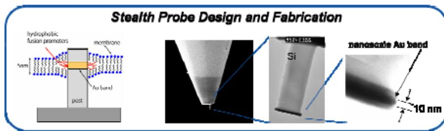
*Stealth electrodes are made with a thin hydrophobic band to insert into the lipid bilayer. Focused ion beam milling followed by metal deposition created the 10-nm thick gold band seen*
