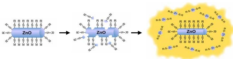
Schematic representation of the thiol encapsulation process of nano-ZnO
