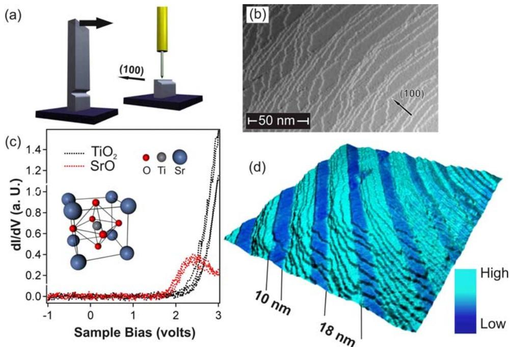
Figure 1(a): Schematic representation of the cleavage process of STO substrates. (b) Topography of the cleaved SrTiO<sub>3</sub>(001) surface. (c) Tunneling spectra taken on TiO<sub>2</sub> and SrO terminated terraces revealing a strikingly different LDOS in the empty electronic states. (d) Rendered 3-dimensional representation of the surface topography shown in (b) color-coded with the simultaneously measured dI/dV conductance map.
