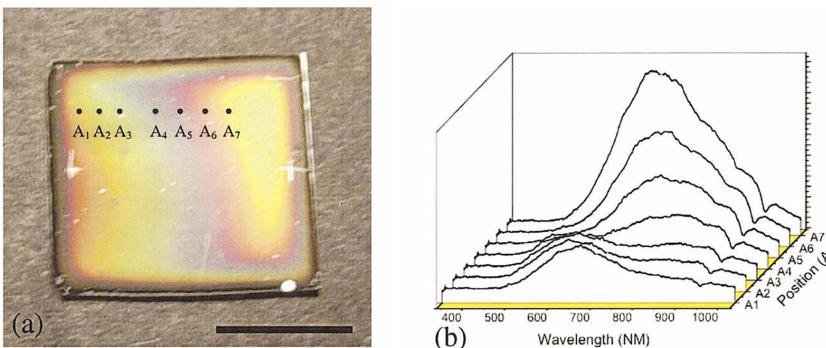
Figure. (Color) Antenna length effect. (a) Interference colors from the random array of MWCNTs. A<sub>1</sub>–A<sub>7</sub> are the selected positions where the length and optical measurements were carried out. Scale bar, 1 cm. (b) Reflected light intensity vs radiation wavelength measured in selected points on the sample shown in (a).
