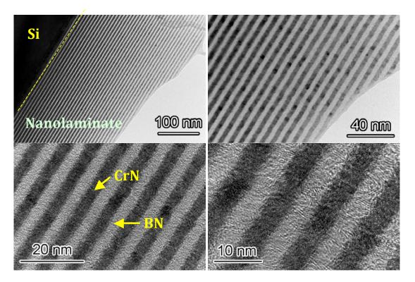
The images are electron microscope pictures of these fine-scale films or nanolaminates. The dark layers are CrN and the light layers are BN. They are deposited in alternating layers using sputter deposition in nitrogen. The layered structure provides additional strength to the individual layers and also provides a more tortuous path for hydrogen diffusion.
