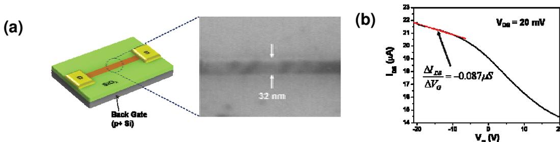
Fig. 3 (a) A back-gated graphene field-effect transistor (GFET) with a 32 nm wide, 0.53 μm long as-exfoliated FLG line as the channel. (b)  $I_{DS} - V_G$  of the GFET, from which the hole mobility is extracted to be  $\mu_h = 1,050 \text{ cm}^2/\text{Vs}$ .
