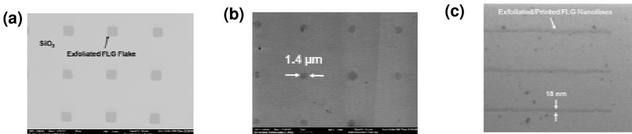
Fig. 2 Representative SEMs of electrically exfoliated/printed few-layer-graphene (FLG) features, which includes (a) 5 x 5 μm squares, (b) 1.4 μm size periodic pillars, and (c) 18 nm wide nanolines.
