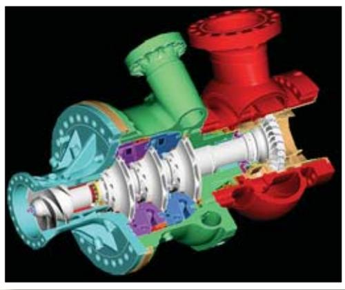
**Impact:** This alloy enables a revolutionary two stage liquid hydrogen turbopump that achieves major objectives of the Integrated High Payoff Rocket Propulsion Technology (IHRPT) Initiative for dramatic increases in thrust-to-weight, reliability and affordability of liquid rocket engines for improved access to space. Additional applications are being pursued with industrial partners, including turbopump housings and large pipes in liquid rocket engines, aircraft wheels and automotive parts.
