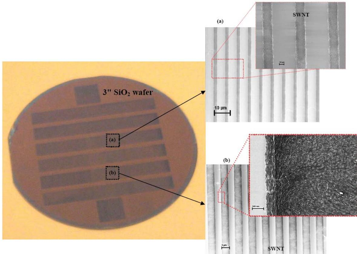
SEM images of the assembled SWNT structures on a 3 inch wafer with pattern widths of (a) 3 μm, and (b) 9 μm structures of assembled SWNTs.
