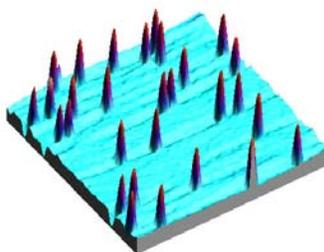
*InAs QDs embedded in an AlGaAs/GaAs structure, with an atomic force microscope image of the uncovered QDs to the right. As the bias current is increased, the shell states fill, and the electroluminescence (EL) from the QDs exhibits*
