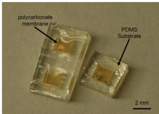
Photograph of sensing devices filled with a solution. The polydimethylsiloxane (PDMS) substrate contains reservoirs which are covered by a semi-permeable polycarbonate (10 nm pore) membrane. The membrane will allow analyte to diffuse into the reservoir and induce nanoparticles aggregation, which is measured by MRI.
