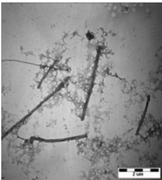
Figure 4.x. MWCNT stabilized in the aqueous phase by Suwannee River NOM.
