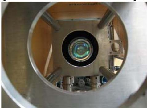
*End-on view of high numerical aperture custom lens system used to trap and image single atoms. Credit: Mark Saffman*
