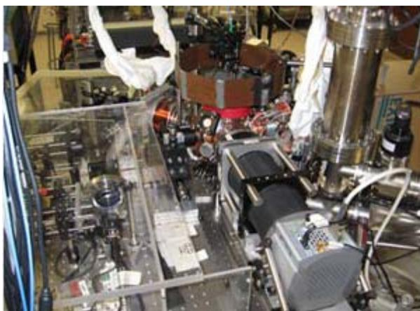
*Mark Saffman's laboratory, showing the vacuum chamber and camera used to detect single atoms. Credit: Mark Saffman*
