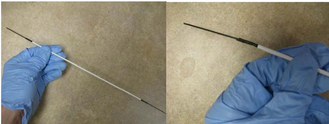
**Figure 1.** Images of the coaxial wire fabricated in the RIT NanoPower Research Labs
