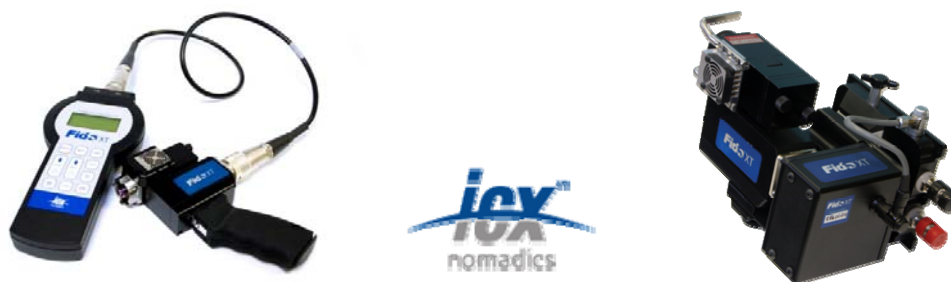
Figure. Fido™ Amplifying Fluorescent Polymer (AFP) Devices for sensing hazardous substances: Hand held version (left panel); Robot integrated version (right panel).
