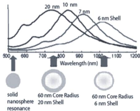
Figure 2.1. Silica core–gold shell nanoshell resonances as a function of the core–shell ratio (courtesy of N. Halas and J. West, Rice University).
