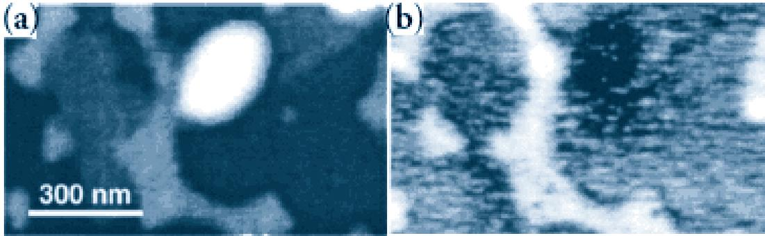
Figure 2.7. (a) Topography of gold patterned on silicon and (b) the corresponding nearfield optical image at 633 nm (courtesy of Keilmann, Max Planck Institut für Biochemie).
