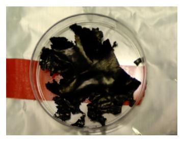
A sample of a film carrying a new material (LiFePO<sub>4</sub>) that could allow quick charging and discharging of lithium ion batteries. Credit: Massachusetts Institute of Technology
